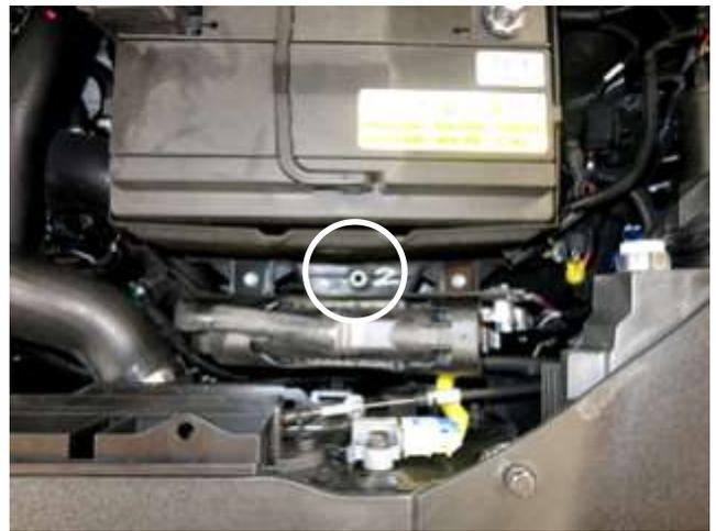
b. Remove the battery hold down bolt and bracket. Then slide the battery as far forward as possible. The bolt and bracket will be reinstalled in step 3q.
