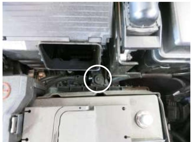
d. Remove the bolt behind the battery that secures the stock air box to the engine compartment.
